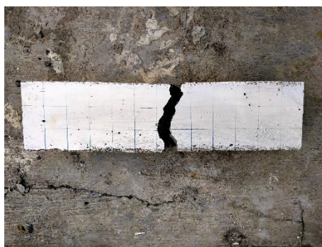
Figure 3. Failure pattern of the 10% sample specimen
