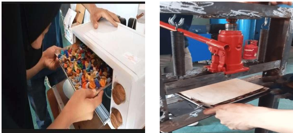
Figure 4 Melting plastic bottle caps in the microwave and fabricating plastic bottle caps using a recycling press
